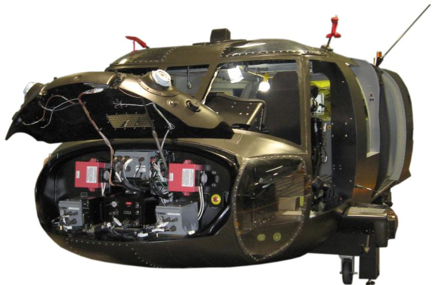
The BHAT-M supports all the critical tasks necessary to train MOS (Military Occupational Specialty) 15N10/30 Avionics Mechanics. Typical 15N training tasks include trouble shooting, isolation of faults and restoration of functionality.
