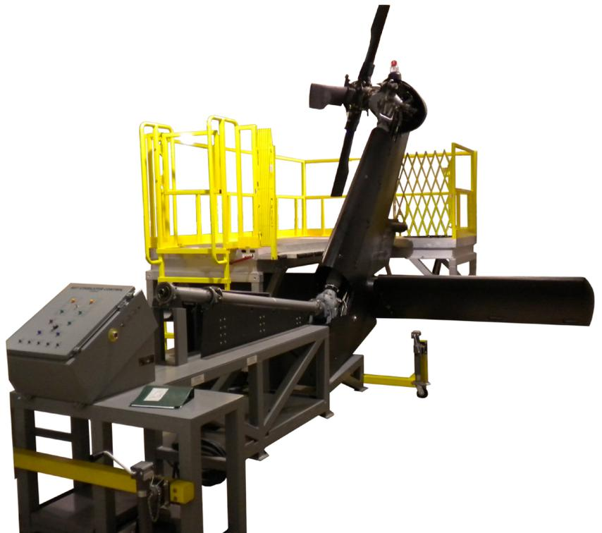
The Student Station is composed of a mock-up tail pylon mounted to a support table to provide stability and safety during operation and includes:
