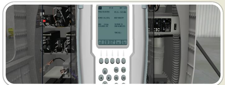
Virtual test set to troubleshoot and diagnose faults. Modeled after tactical test set, MBRAT enables students and instructors to perform Remove and Replace Tasks, component troubleshooting, along with the use of simulated virtual aircraft test sets.
